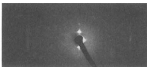
FIGURE 3 X-ray diffraction pattern of the substance with n = 11 at 90^{\circ}\text{C} , magnetic field oriented, arrow indicates field direction.
